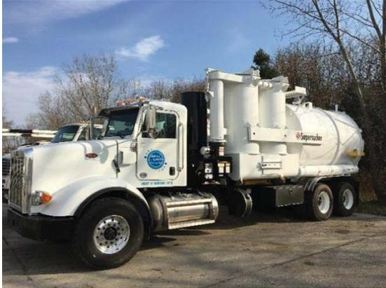
GLPV is happy to introduce the latest addition to its already-impressive fleet of trucks: the 2017 Supersucker® Industrial Vacuum Loader by [Super Products](#). Its high-power airflow moves solids, liquids, sludge, and slurries through suction lines up to 8" in diameter, making it ideal for industrial waste removal, bulk material delivery, and environmental cleanups.
