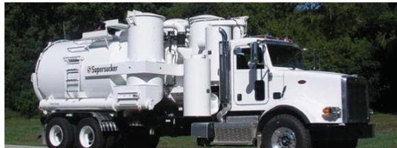
Driven by customer demand, Great Lakes Power Vac has added to its already-impressive fleet of trucks. We are excited to announce the addition of a new Supersucker® Industrial Vacuum Loader, one of the most popular and requested vacuum trucks in the industry. Offering high-power airflow to convey solids, liquids, sludge, and slurries through suction lines up to 8" in diameter, the Supersucker® is ideal for industrial waste removal, bulk material recovery, and environmental cleanups.
